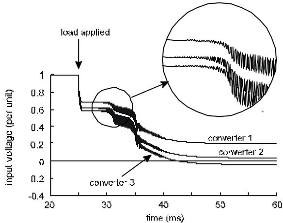
Figure 4: Results of Pspice simulation, damping components omitted
