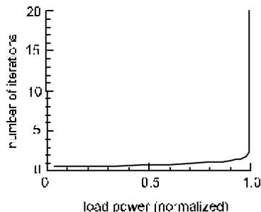
While convergence of the software and stability of the system are not exactly equivalent, they are strongly related. Provided power transfer is kept at or below about 95% of the theoretical peak value, stable operation should result.
