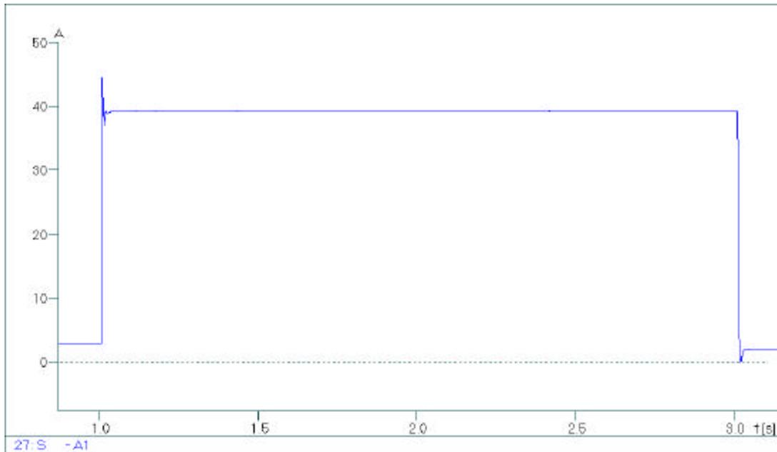
**Figure 6.10 Output current of shore power supply without current limiting**
