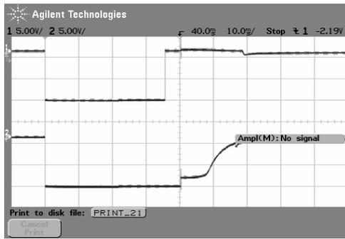
Channel (1): Command signal to power the  $4\ \Omega$  load
