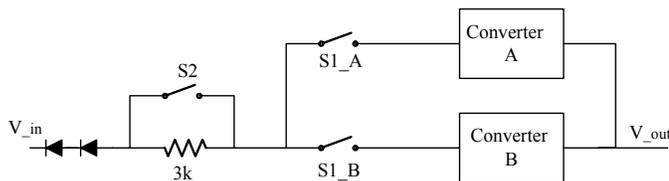
Fig. 4. Science node converters input circuit configuration
