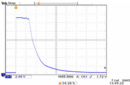
Fig. 12. Startup power supply output when firing a converter at -8 kV (inverted)
