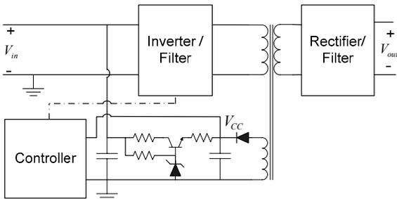
Fig. 6. Converter startup circuit 2
