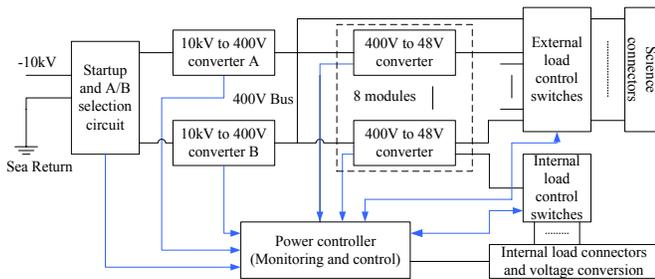
Fig. 3. Science node power system block diagram
