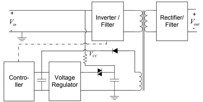
Fig. 7. Converter startup circuit 3
