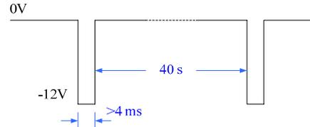
Fig. 10 The ideal output of startup power supply when a converter is being started
