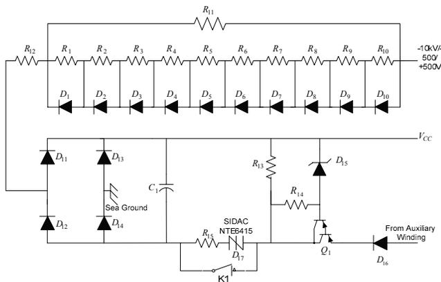
Fig. 9. Startup power supply designed for 10 kV to 400 V dc converters
