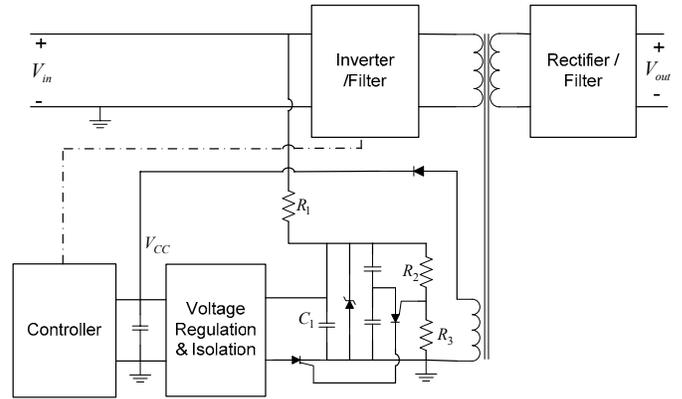
Fig. 8. Converter startup circuit 4
