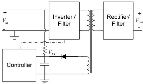
Fig. 5. Converter startup circuit 1
