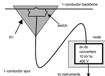
Fig. 2. Layout of science node connection
